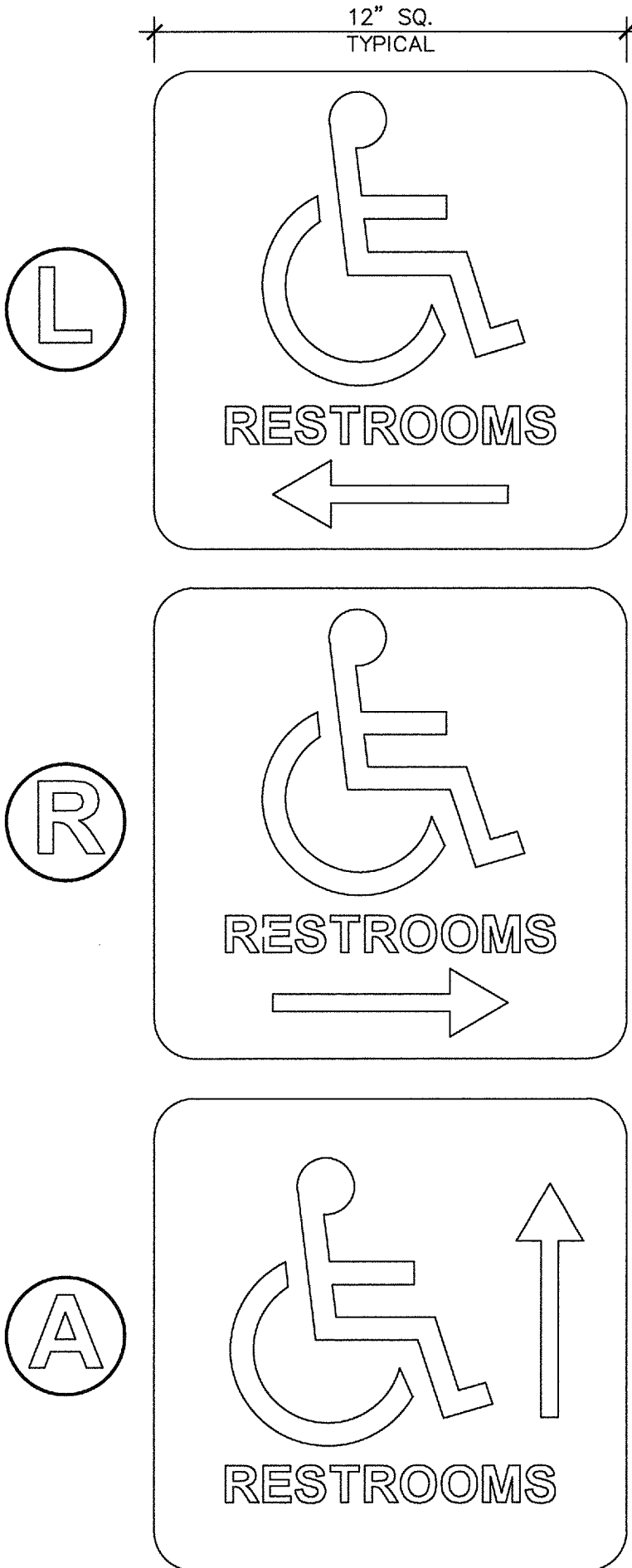
16 ACCESSIBLE RESTROOM DIRECTIONAL SIGNAGE A1.05 ADA100-04 SCALE: 1" = 1'-0"
