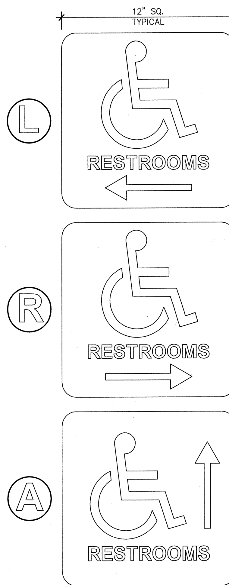
6 ACCESSIBLE RESTROOM DIRECTIONAL SIGNAGE ADA100-04 SCALE: 1' = 1'-0"
