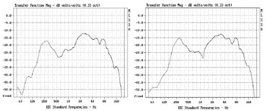
Note: The wide band frequency response is derived using MLS methods
