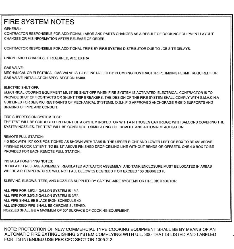
NOTES - FIELD PIPE DROPS AS SHOWN SLEEVING, ELBOWS, TEES, AND NOZZLES SUPPLIED BY CAS - RELOCATE NOZZLES IF FLOW PATTERN IS BLOCKED BY SHELVING,
