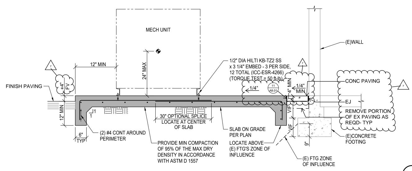
SECTION AT MECH UNIT SLAB ON GRADE
